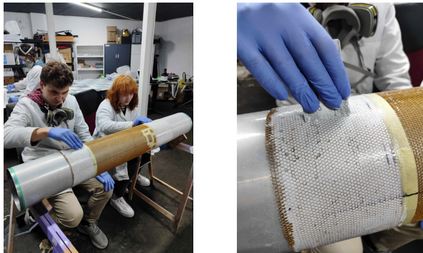
FIGURE 3. Hand made electronics fuselage. Team members winding subsequent layers around an aluminium tube that works as a mould. Honeycomb and micro-balloons (white regions) are shown.
