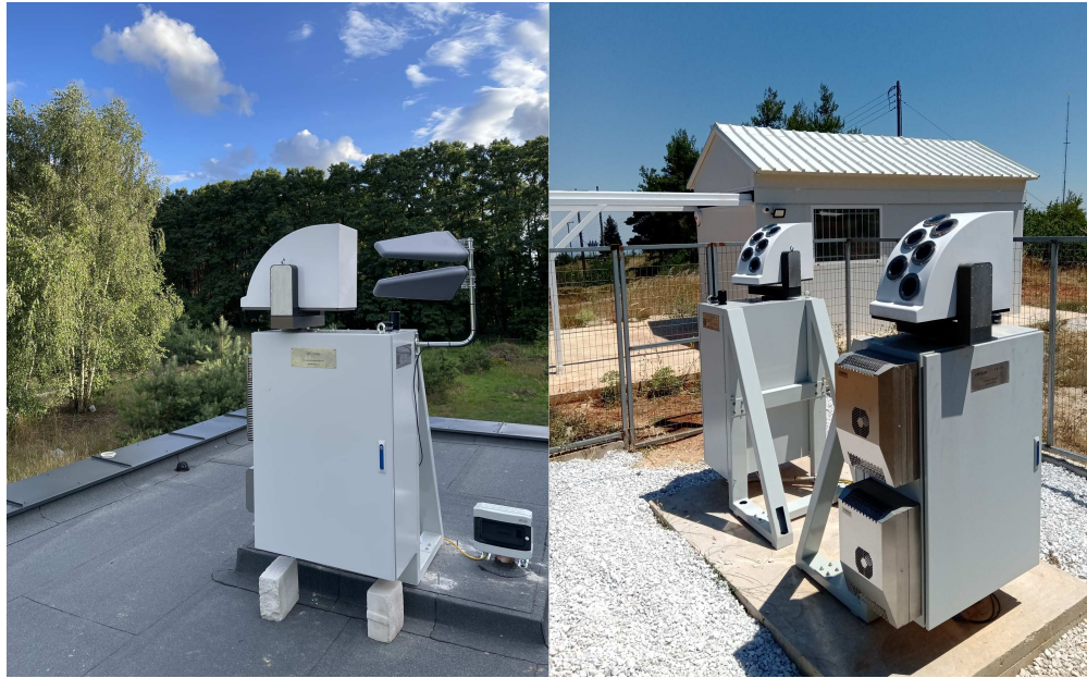
FIGURE 1. OpticNode station Alpha-1 (left), OpticalFence station 1-A2 (right, in the foreground) and OpticNode Alpha-2 (right, behind the OF station).
