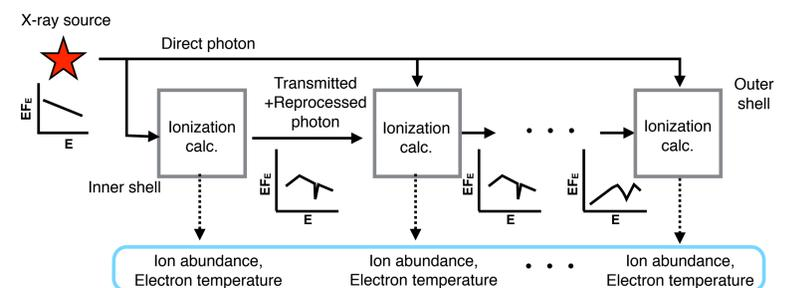
Fig.3 Schematic view of the ionization calculation
