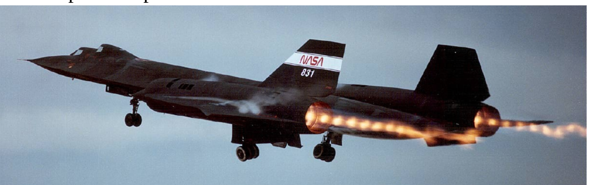
Figure 2 : Top- Formation of shock diamond during takeoff of an SR-71 aircraft ( http://www.nasa.gov/centers/armstrong/ ). Bright knots are the location of shock due to recollimation of flow under external-medium pressure. Bottom- Idealized steady-state structure of a slightly under-expanded supersonic jet. The red lines represent the incident and reflected shock. Black streamlines follow the oscillating flow path of the jet gas (Norman & Winkler, 1985).
