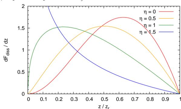
Distribution of dissipated energy flux along the jet. For  $\eta \gtrsim 1.3$  the flux peaks at the jet origin.
